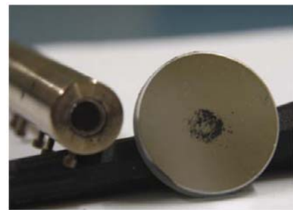
Figure 13. Soot deposits on optical surfaces.
