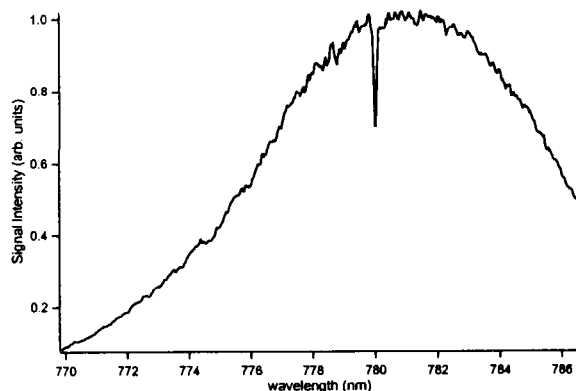
Figure 3 Spectrum of Rb aspirated into a flame obtained by using the spectrally broad Ti:sapphire laser beam and a scanning monochromator.
