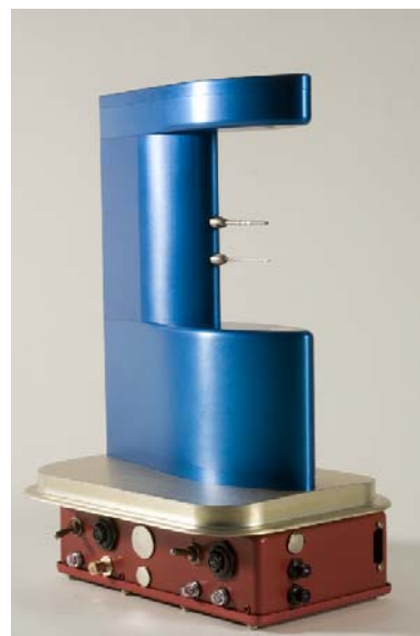
Figure 1. Photograph of the Southwest Sciences' VCSEL hygrometer showing the electronics box (red), aperture plate (gold), and pylon (blue). Light is passed 25 times between mirrors at the front of the pylon. The electronics box resides inside the aircraft immediately below the pylon.
